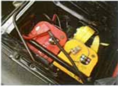
90's twin batteries: red for all the vehicle systems; yellow to power the computer
